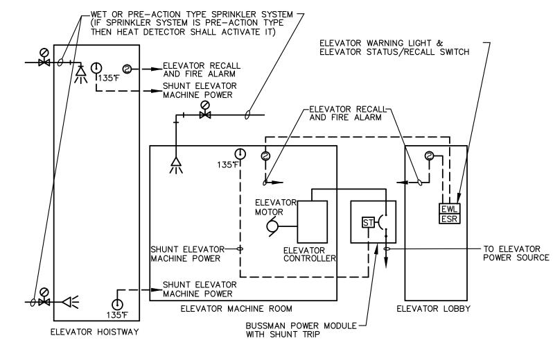
ELEVATOR FIRE CONTROL & ALARM DETAIL N.T.S.
